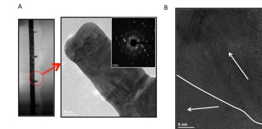
TEM shows that NPs completely fuse without any voids or gaps.
