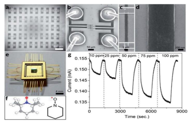
SEM images setup for assembled SWCNT array devices. (e) An optical image of wafer scale sensor devices. (f) Chemical structure of TEMPO molecules. (g) Real-time current changes as a function of conc.  $H_2S$  gas at 10, 25, 50, 75 and 100 ppm for the functionalized SWCNT sensor.
