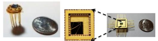
**Our Chemical Hydrogen Sulfide (H2S) Sensors**
