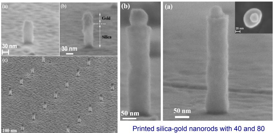
Printed hybrid silica-gold nano rods over a large area.
